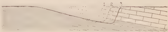
FIG. 63. — Unsymmetrical valley formed as a result of the dip of the rock.
